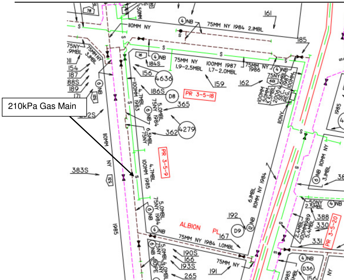
Figure 7 – Jemena Natural Gas Infrastructure (Kent Street)
